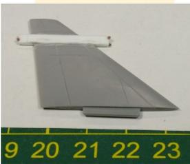
Next, styrene stripe was cut and shaped to represent the chaff and flare dispensers installed under the rear fuselage (Photo 3).
