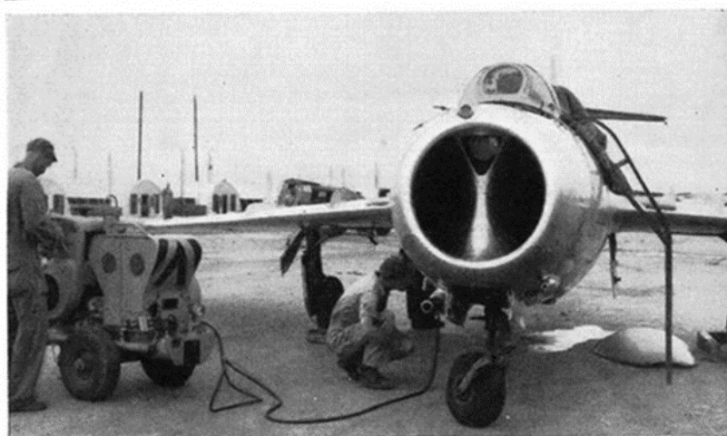
MIG BEFORE TAKEOFF shows characteristic chunky lines, broken by bulges for guns and ejection chutes. Pins protruding from wing between fences and ahead of cockpit are visual landing-gear indicators. At left of windshield is shielded pitot.
