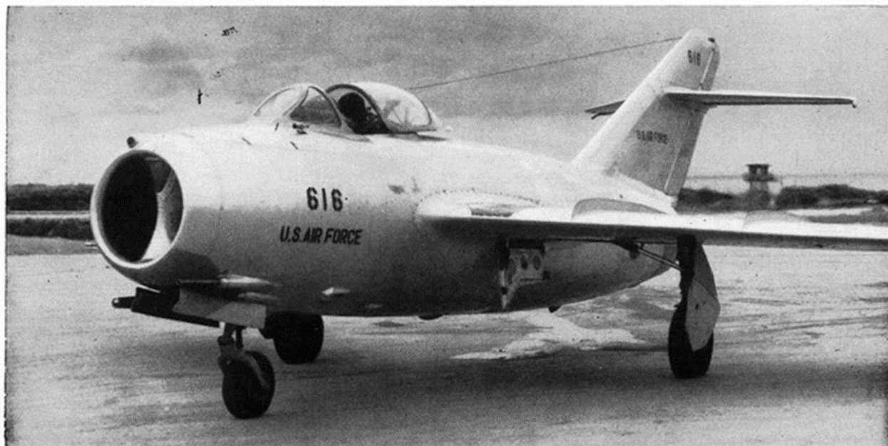
MIG NOSE uses waste space in duct splitter for landing light. Gun camera mounts over cowl inlet; cowl panel for access lies on ground under left wingroot. View shows anhedral droop of swept wings, circular fuselage cross-section.
