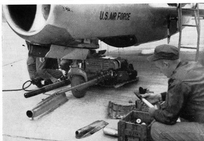
MIG ARMAMENT pack lowers from fuselage on four cables for access. Fairings on ground cover exposed barrels. Larger cannon (37-mm.) mounts recoil spring and blast tube externally. Panel under nose probably is steel, protects against gunblast.
